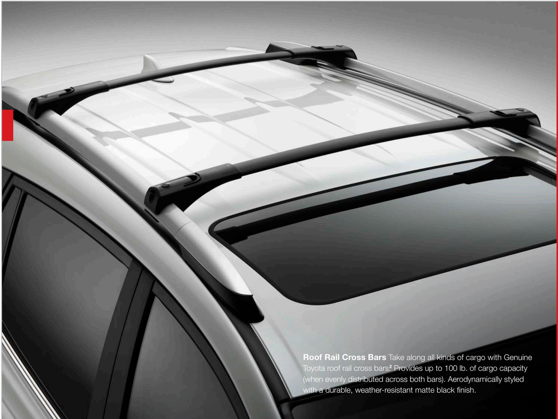
**Roof Rail Cross Bars** Take along all kinds of cargo with Genuine Toyota roof rail cross bars.<sup>2</sup> Provides up to 100 lb. of cargo capacity (when evenly distributed across both bars). Aerodynamically styled with a durable, weather-resistant matte black finish.
